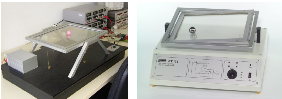
Figure 3: Ball-on-Plate (left: prototype of Harz University; right: industrial reproduction) (Kramer & Braune, 2001; GUNT Gerätebau GmbH, 2007)
