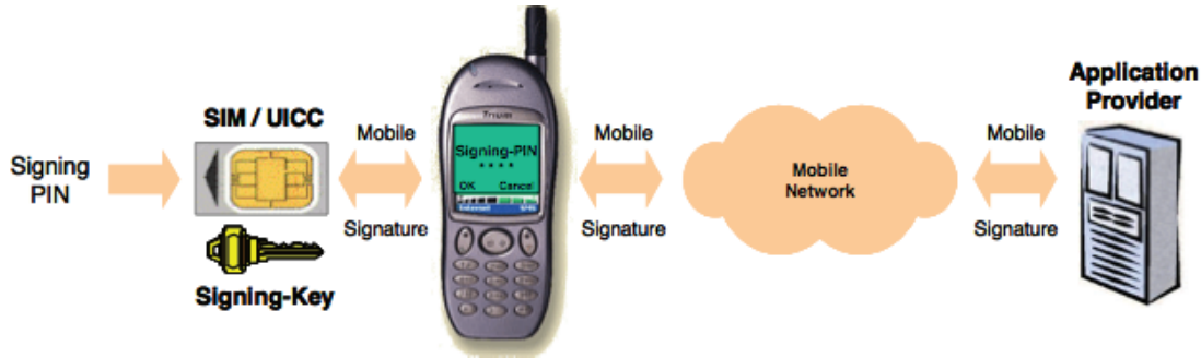
Figure 2: Typical mobile smartcard implementation. (ETSI, 2003a)
